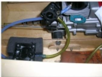
Run a water line from your water pickup (this should be a pickup that is constantly in the water such as a rudder blade pickup or transom mounted pickup, NOT a prop blast pickup) to the pump's inlet and another line from the pump's outlet to your boat's engine. From the engine the water might exit the boat or go to a tuned pipe system, depending on components used.
